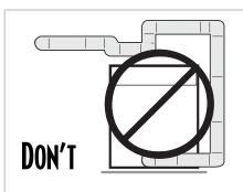
Use longer than necessary duct runs with many elbows.
